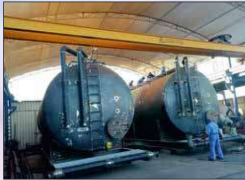
Skid Mounted Recirculation Storage tank
